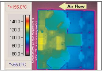
Figure 8: Thermal plot of converter at 17 amp load current (204 Watts) with 55°C air flowing at the rate of 200 LFM. Air is flowing across the converter from output to input (nominal input voltage).
