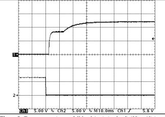
*Figure 9: Turn-on transient at full load (resistive load) (10 ms/div). Input voltage pre-applied. Top Trace: Vout (5V/div). Bottom Trace: ON/OFF input (5V/div)*
