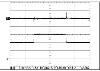
**Figure 11:** Output voltage response to step-change in load current (50%-75%-50% of Iout(max);  $dI/dt = 0.1A/\mu s$ ). Load cap:  $15\mu F$ ,  $450 \text{ m}\Omega$  ESR tantalum and  $1\mu F$  ceramic. Top trace: Vout (1V/div), Bottom trace: Iout (5A/div).
