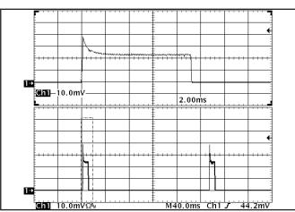
**Figure 18:** Load current (10A/div) as a function of time when the converter attempts to turn on into a  $1 m\Omega$  short circuit. Top trace (2ms/div) is an expansion of the on-time portion of the bottom trace.
