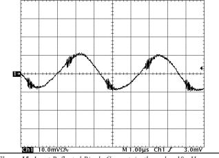
**Figure 15:** Input Reflected Ripple Current,  $i_{S'}$  through a 10  $\mu$ H source inductor at nominal input voltage and rated load current (5 mA/div). (See Figure 13)
