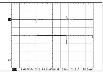
**Figure 12:** Output voltage response to step-change in load current (50%-75%-50% of Iout(max):  $dI/dt = 5A/\mu s$ ). Load cap:  $480\mu F$ , 15 m $\Omega$  ESR tantalum and  $1\mu F$  ceramic. Top trace: Vout (1V/div), Bottom trace: Iout (5A/div).
